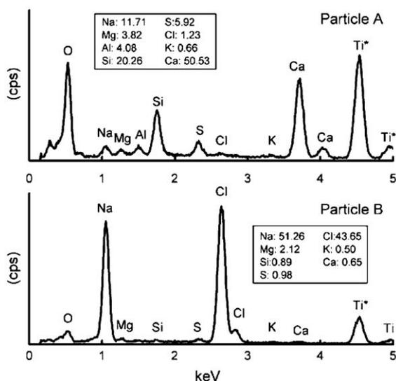
Fig. 2. SEM photograph of collected particles (the particles were collected on 9 March) and the X-ray spectra of a mixture particle of mineral dust and sea salt (particle A) and a sea salt particle (particle B). Data in the frames in each spectrum are the raw relative weight ratios of detected elements in the particles.
