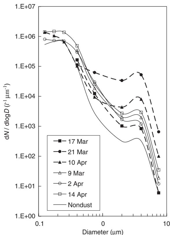
Fig. 6. 1-h average particle number–size distributions per liter air masses measured by the particle counters when particle collection was carried out. A case of nondust period distribution, which was recorded around 0630 on 9 May, is added for comparison. The concentrations in the size range of 0.3–0.5  $\mu\text{m}$ , which is overlapped by the two counters, are averages of data from the two counters.
