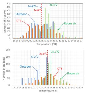
Figure 2: CTS, Room air temperature, and Outdoor temperature in Sapporo (Above: 2009-12, bottom: 2014)
