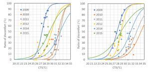
Figure 5: CTS and the ratio of discomfort in Kumamoto (Left: at the window side, Right: at the corridor side)
