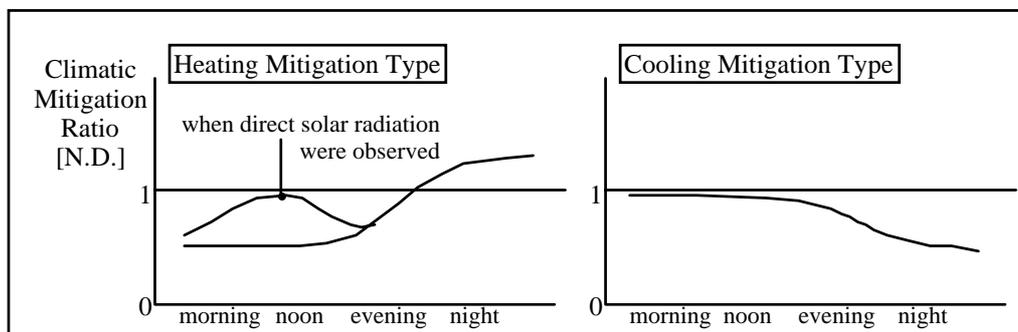
Fig. 9: The semi-outdoor spaces expressed as heating mitigation and that as cooling mitigation
