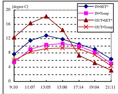
Fig. 1: Air temperature and SET\* at Imabari (Aug. 10) Fig. 2: Air temperature and SET\* at Imabari (Jan. 11)
